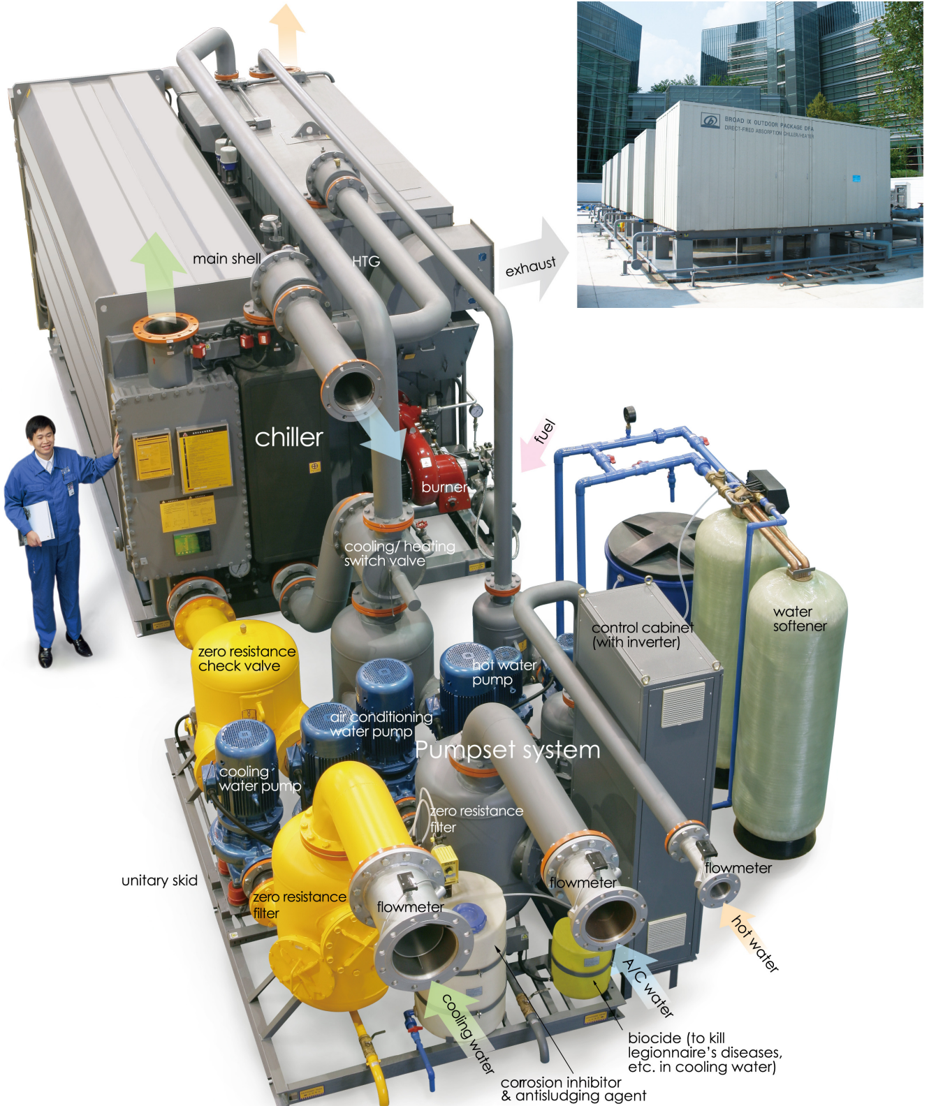
Exhibit 2: BROAD's Modular Package Air Conditioning System
