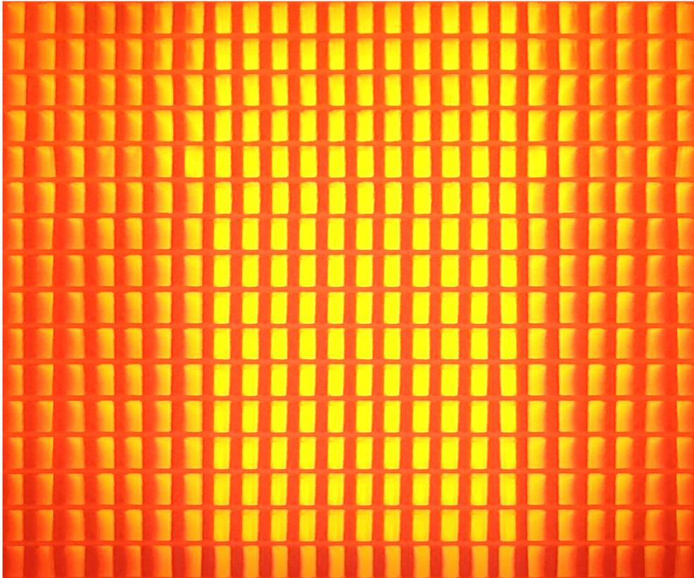
Bcore slab brazing technology: two steel plates are fused to each other by an array of extremely thin core tubes with copper foil at a 1100°C brazing process.
