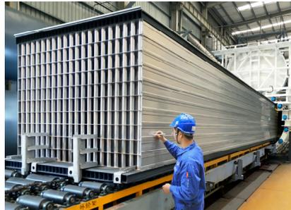
The hot air copper brazing oven: 36 m<sup>3</sup> of Bcore slab/oven, yearly yield: 400 thousand to 2 million m<sup>2</sup>; only one technician is needed for each shift. Note: Due to confidentiality, it is not authorized to take pictures of the oven.
