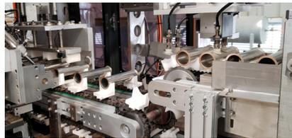
Pre-brazing sheet metal processing line: 800 thousand m<sup>2</sup>/line; intelligent manufacturing; three technicians for each shift.
